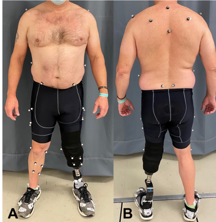
Figure 1. Placement of full-body markers on a PDU from the anterior and posterior (A and B respectively).
