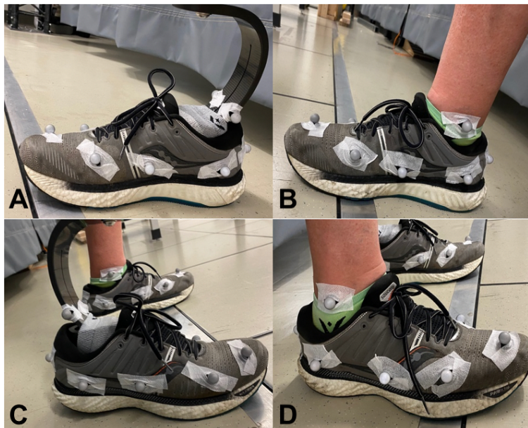
Figure 2. Placement of foot and ankle markers on a PDU showing medial views of both feet (A and B) and lateral views of both feet (C and D).
