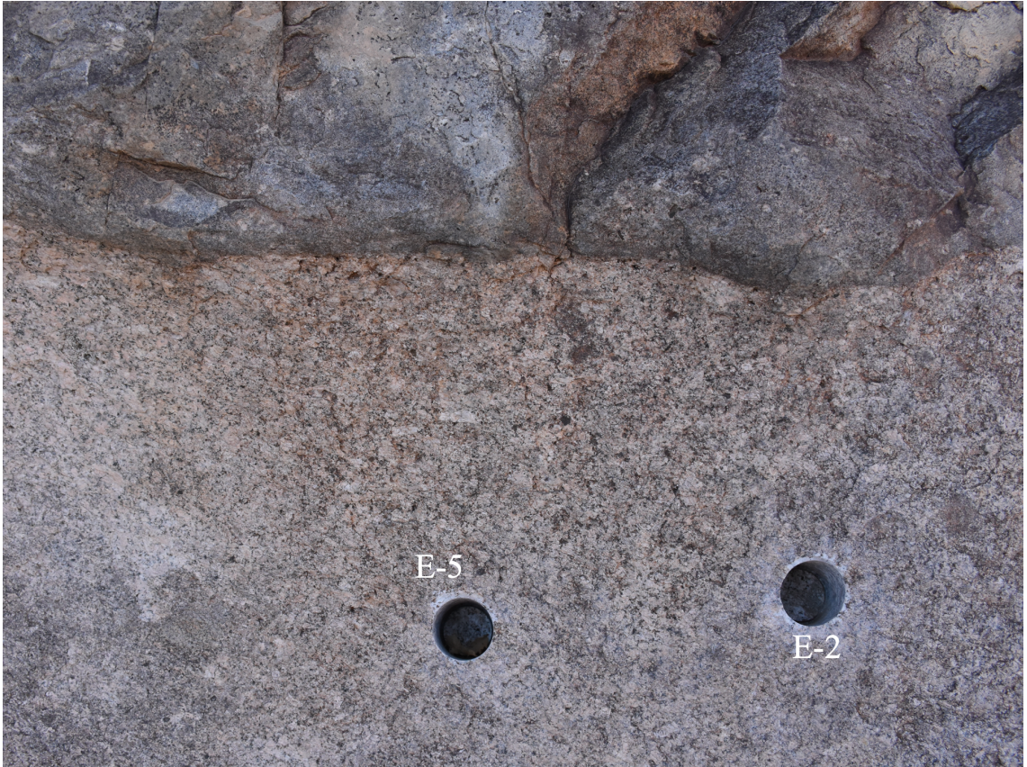
Figure 3: Sample locations for E-5 and E-2, underneath the BFE. Note that directly underneath the enclave, we can observe an oriented fabric in the alkali feldspars, parallel to the base of the BFE. The sampling locations of E-5 and E-2 aim to capture this fabric.
