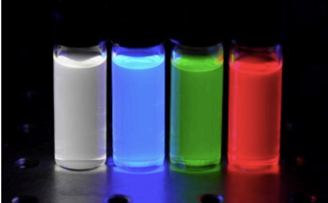
Figure 1.2 CdSe nanocrystals of various sizes, from ultrasmall white light emitting to 7 nm red emitting QDs, used to demonstrate size-dependent quantum confinement.
