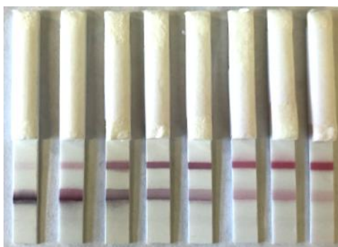
Figure B.7: Representative tests of the standard curve with 50 \text{ ng mL}^{-1} CAA (far left) to 0 \text{ ng mL}^{-1} CAA (far right).
