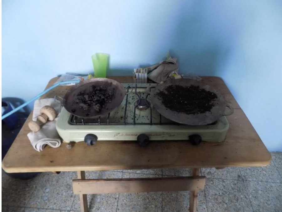
Figure 4.6 Soil Samples Prior to Heating at Lab in Café Yaxha, Flores, Guatemala
