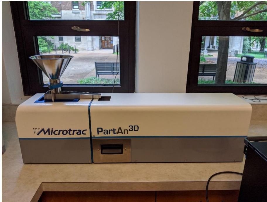
Figure 4.9 PartAn 3D Analyzer in the Ancient Artifacts Lab at Vanderbilt University
