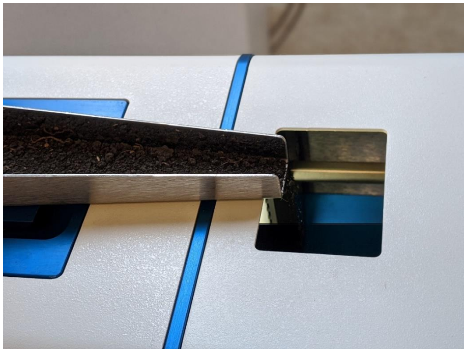
Figure 4.10 Soil Particles Passing through the Vibrating Tray into the Analyzer to be Photographed
