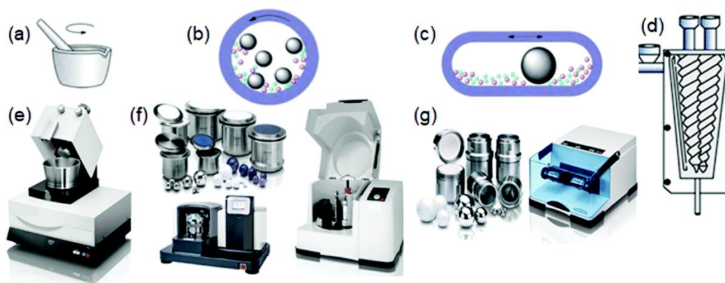
Figure 1. Schematic illustration of mechanochemical equipment. (a) mortar and pestle, (b) planetary mill, (c) shaker and (d) extruder. Images of the instruments for mechanochemical synthesis: (e) mortar grinder, (f) planetary mills with equipment and (g) mixer mill with equipment (reproduced with permission of the RSC)
