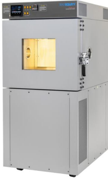
Fig. 4-3. Test Equity model 140 temperature chamber.
