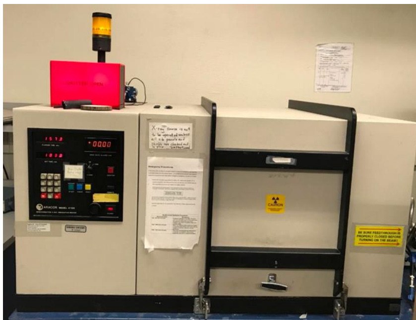
Fig. 5-2. 10-keV ARACOR 4100 X-ray irradiator.
