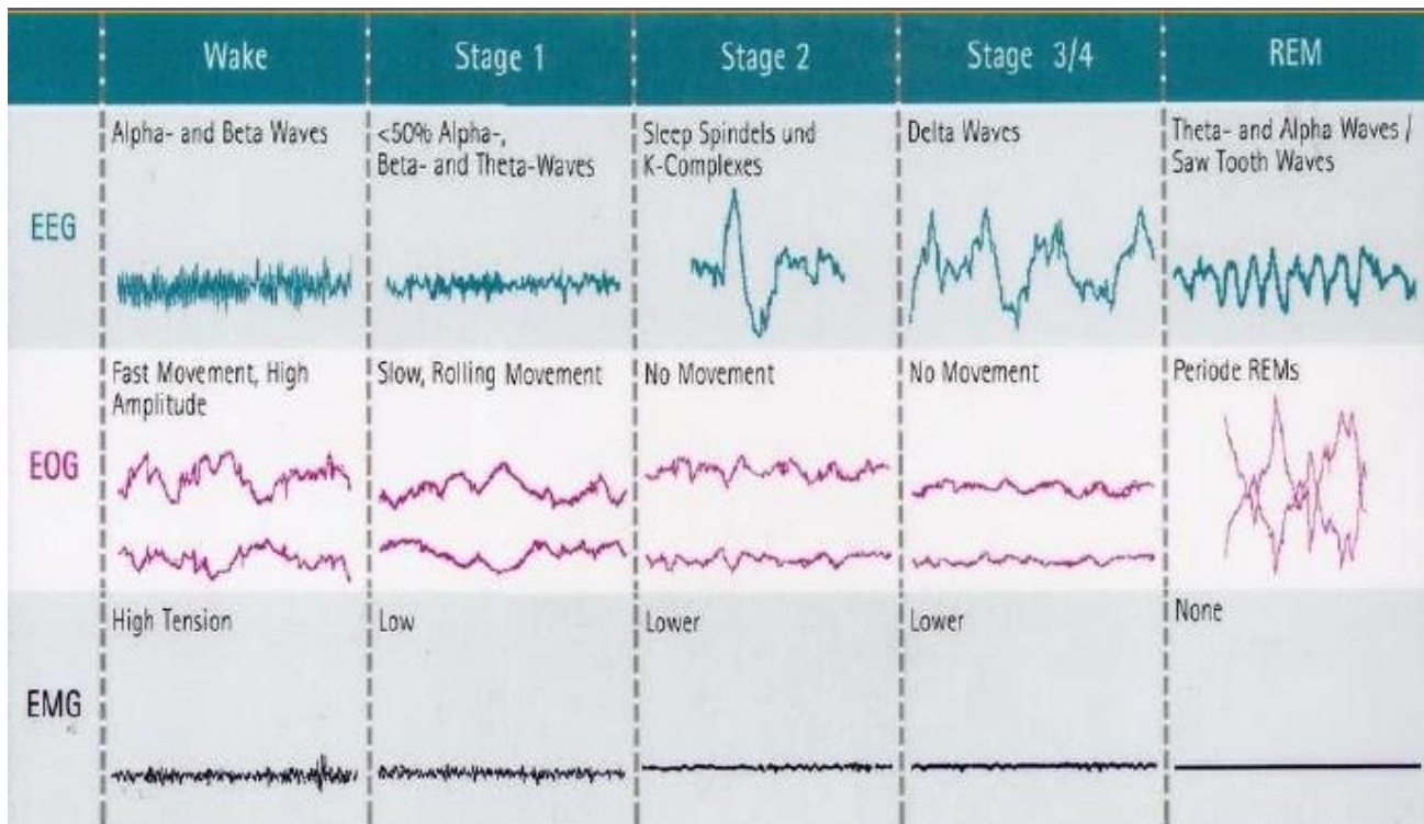
Figure 2. Sleep stage summary. The EEG channel describes brain activity, EOG channel describes eye activity, and EMG channel describes muscle movement. 47
