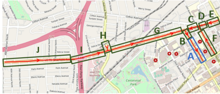
Figure III.12: Road segment for congestion event 10 in Table III.1. The source road of congestion is road segment ‘A’. Following the congestion at the source road segment, the congestion propagates to the 1st (‘B’), 2nd (‘C’, ‘G’) and 3rd hop (‘D’, ‘E’, ‘F’, ‘H’, ‘I’, ‘J’) incoming neighbors respectively.
