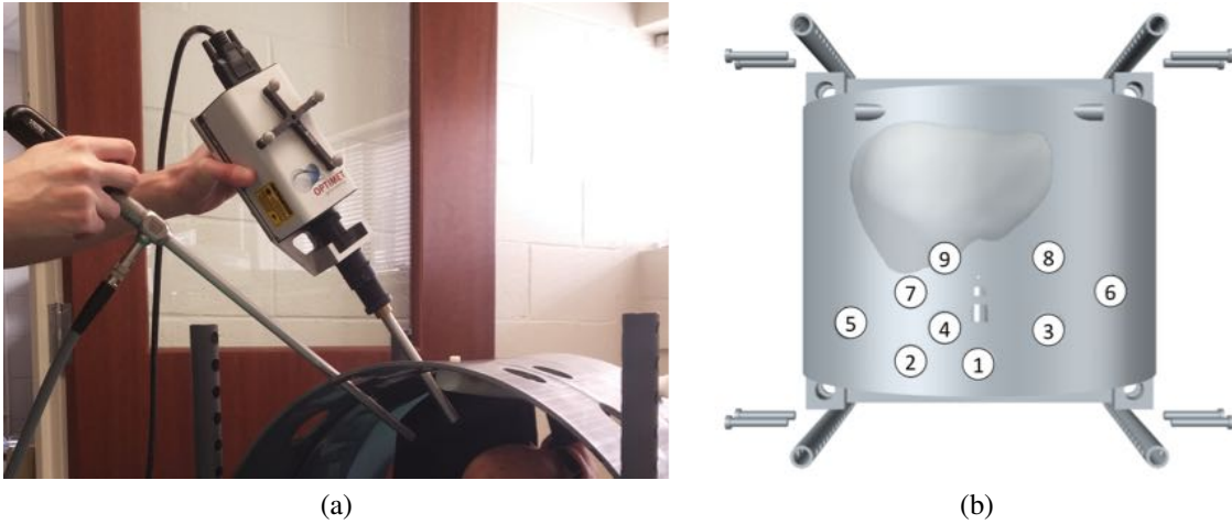
Figure A.4: (a) Experimental setup of intraoperative data collection using the conoprobe. The conoprobe laser beam can be guided by a laparoscope. (b) Placement of the nine access ports in the abdominal frame. Port 1 is located at the umbilicus.
