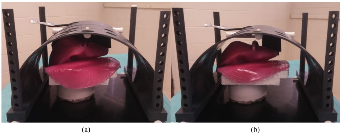
Figure A.2: Inferior view of the soft-tissue liver phantom in the laparoscopic abdominal frame (a) with support, and (b) without support from the falciform and right triangular ligaments, simulating right lobe mobilization. Note the deformation that has occurred following removal of the ligament attachments to the liver.
