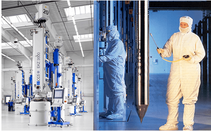
Figure 1.2. (left) A commercial boule growing system from PVATePla (right, image used with permission) a boule of Si to be cut into wafers (from waferpro.com, image used with permission).
