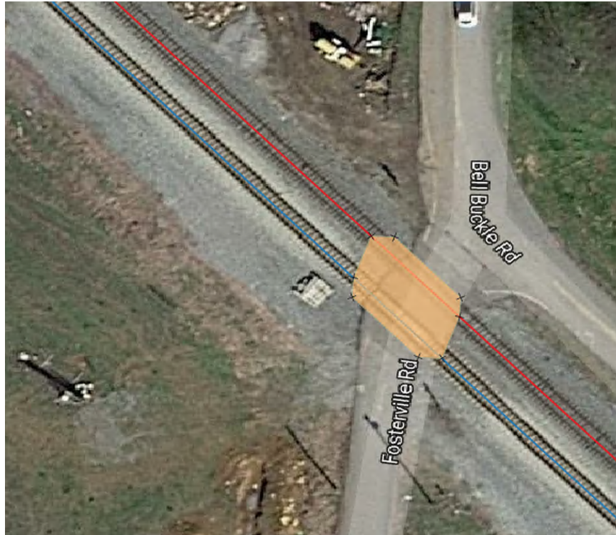
Figure A.2: A single grade crossing boundary delineated by the orange shaded area and overlaid on a satellite imagery basemap. The tracks at this location are shown by the blue line (main line track) and red line (siding track).
