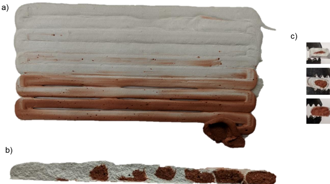
Figure 20 – Printed geometry showing the first material, the transition stage, and the second material from an a) overhead view, b) overall cross-sectional view, and c) individual cross sections
