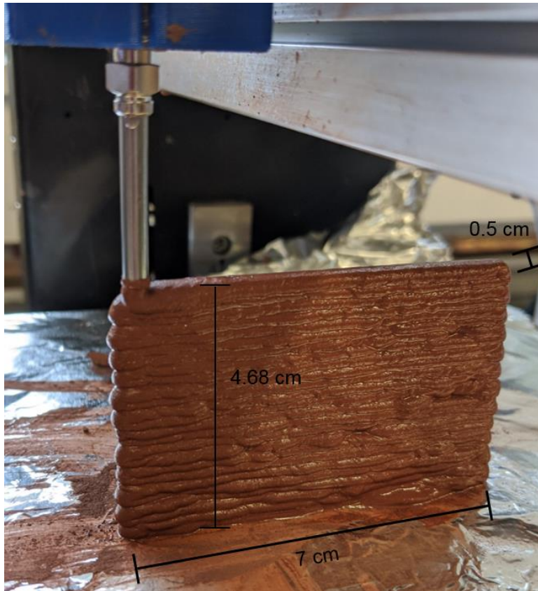
Figure 32 – Second high aspect ratio print, immediately before collapse
