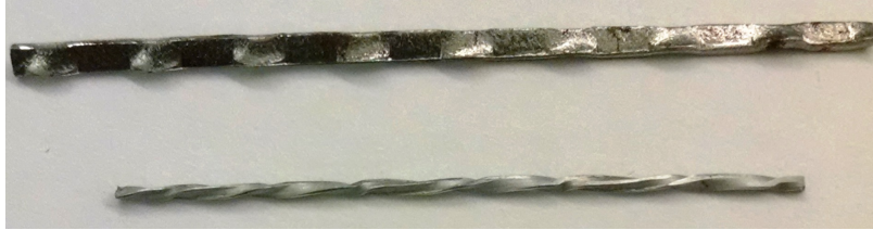
Figure 3.4: Two types of fiber surface deformities: crimping (top) and twisting (bottom).
