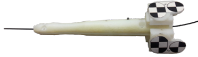
Figure 3.2: Cochlear Inspection Tool comprised of a 1mm flexible fiberscope with 10,000 imaging fibers, a user handle and optical tracking markers.
