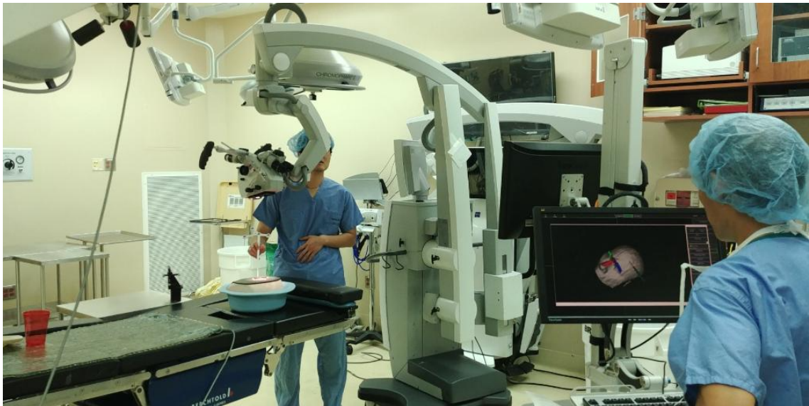
Figure 6.3: The experiment settings in the operating room (OR). The phantom is placed under the surgical operating microscope. A tracked rigid body tracking star is attached on the microscope to permit tracking of the microscope position. The monitor displays the interface of image-to-physical registration in a neuronavigation guidance system.
