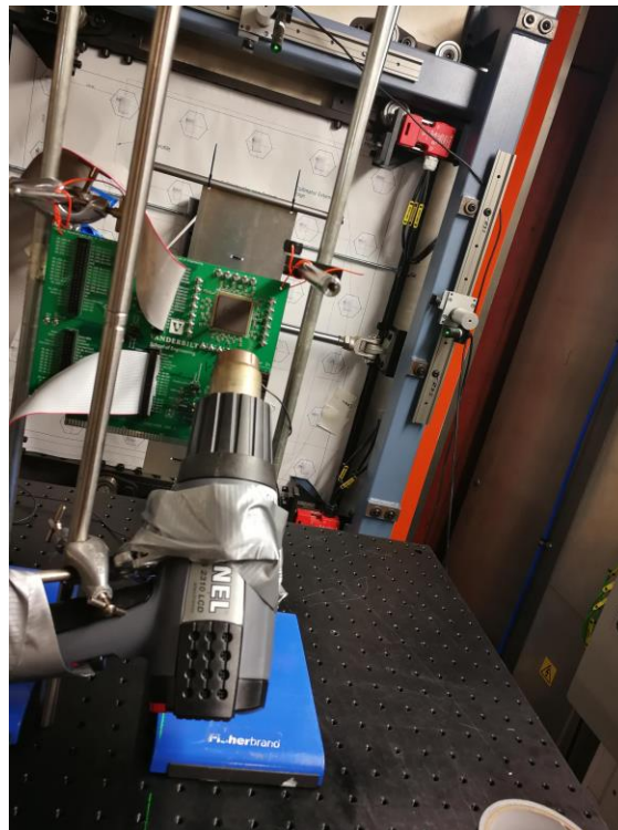
Fig. 2-4 Typical test setup of the neutron tests
