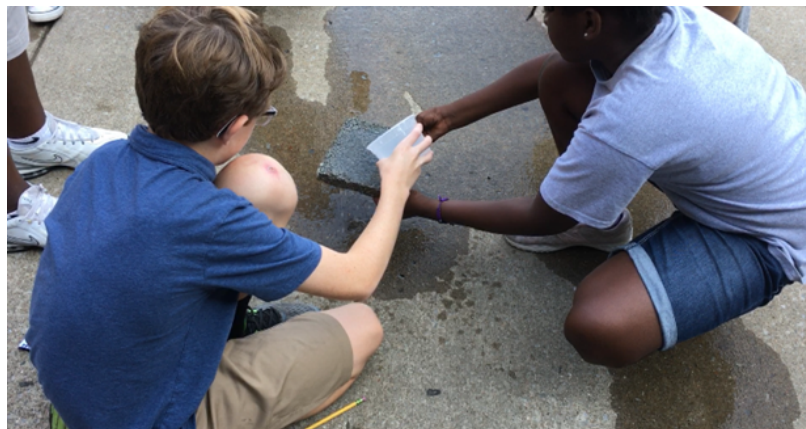
Figure 5.2: Students conducting investigations on the absorbency of different surface materials (image showing the permeable concrete that can be used for a parking lot to reduce standing water and runoff)
