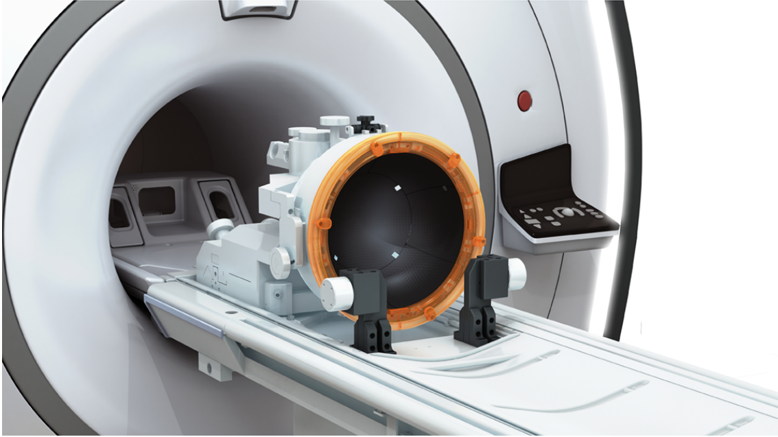
Figure 2.2: The Insightec ExAblate 4000 ("Neuro") is a commercial transcranial MRgFUS system used in the US. It uses a 1024-element phased array ultrasound transducer operated near 650 kHz with a focal length of 15.0 cm and a diameter of 30.0 cm ( f/0.5 ), which enables targeting of deep brain regions in humans with high spatial specificity and with concurrent MRI guidance. Currently, it is the only FDA-approved clinical device available for performing MRgFUS ablative thalamotomy in humans. Image courtesy of Insightec.
