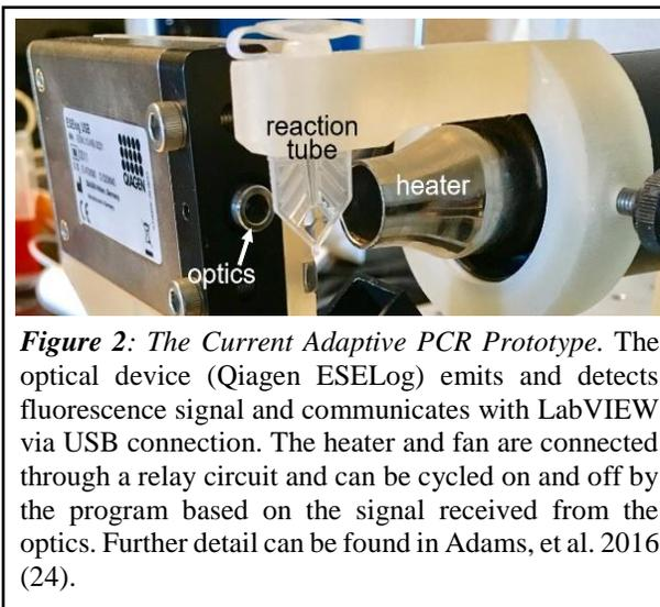
based on the actual state of the DNA, Adaptive PCR achieves optimum thermal cycling even if the sample contains unexpected background contaminants.
