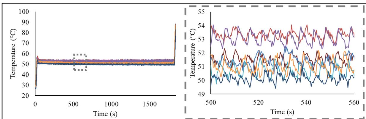
**Figure 4:** *Thermocouple-Monitored Molecular Beacon Holds.* Seven 30-minute trials of reverse transcription temperature holds by the Adaptive PCR instrument using the molecular beacon indicator. The larger graph shows the full 30 minutes, including less than one minute on each end to show initial fitting and transition into cycling. The zoomed-in graph shows intra-trial variation during a one-minute period.
