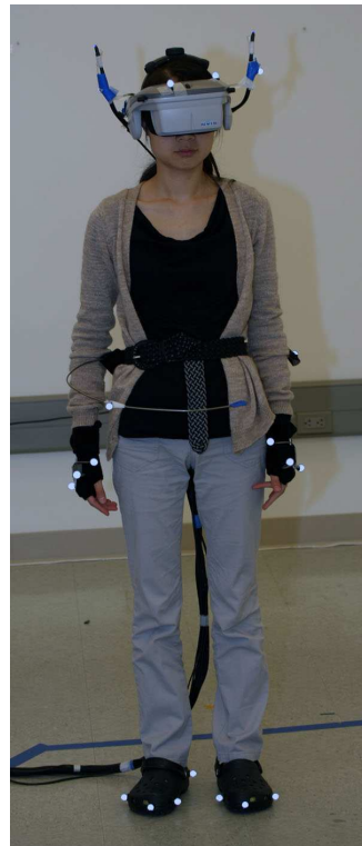
Figure IV.4: This figure shows a person wearing the HMD and motion capture components (left), motion capture components along (top right) and the avatar models used for the self-avatar (bottom right).
