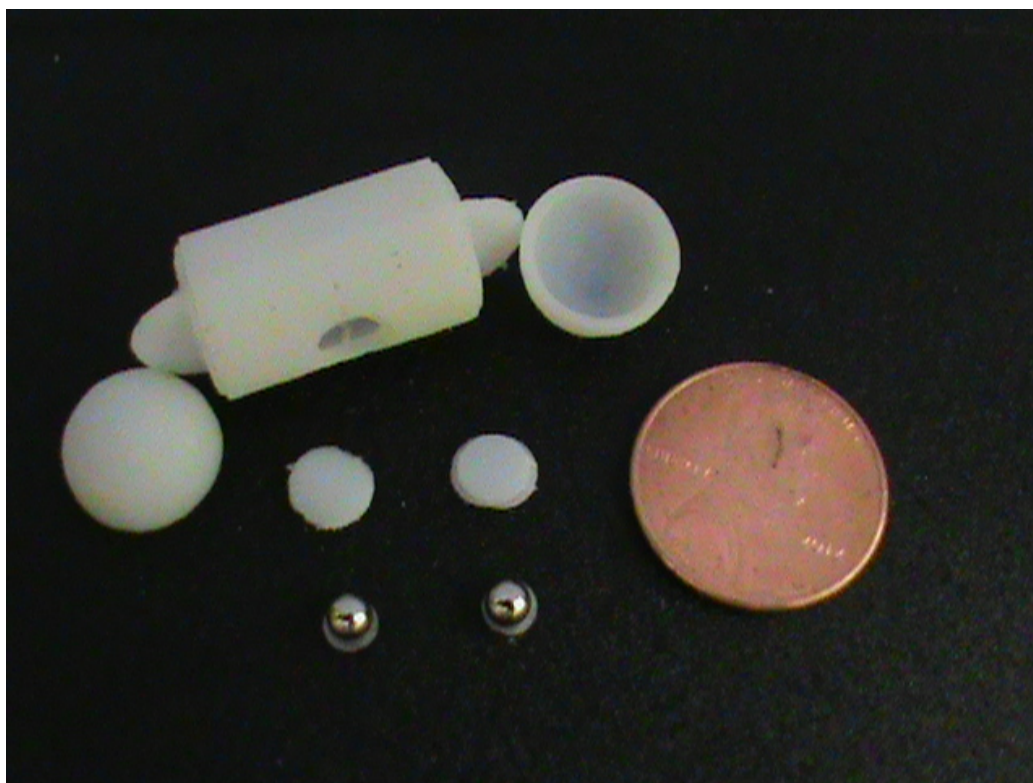
Figure 4.9: Various components of second generation internal reaction capsule including capsule body (12mm diameter by 32mm length), dividing wall (1mm thick), magnetic spheres (3.2mm diameter) and ferromagnetic rings (4.173 mm OD, 1.27mm ID, 0.1mm thick).
