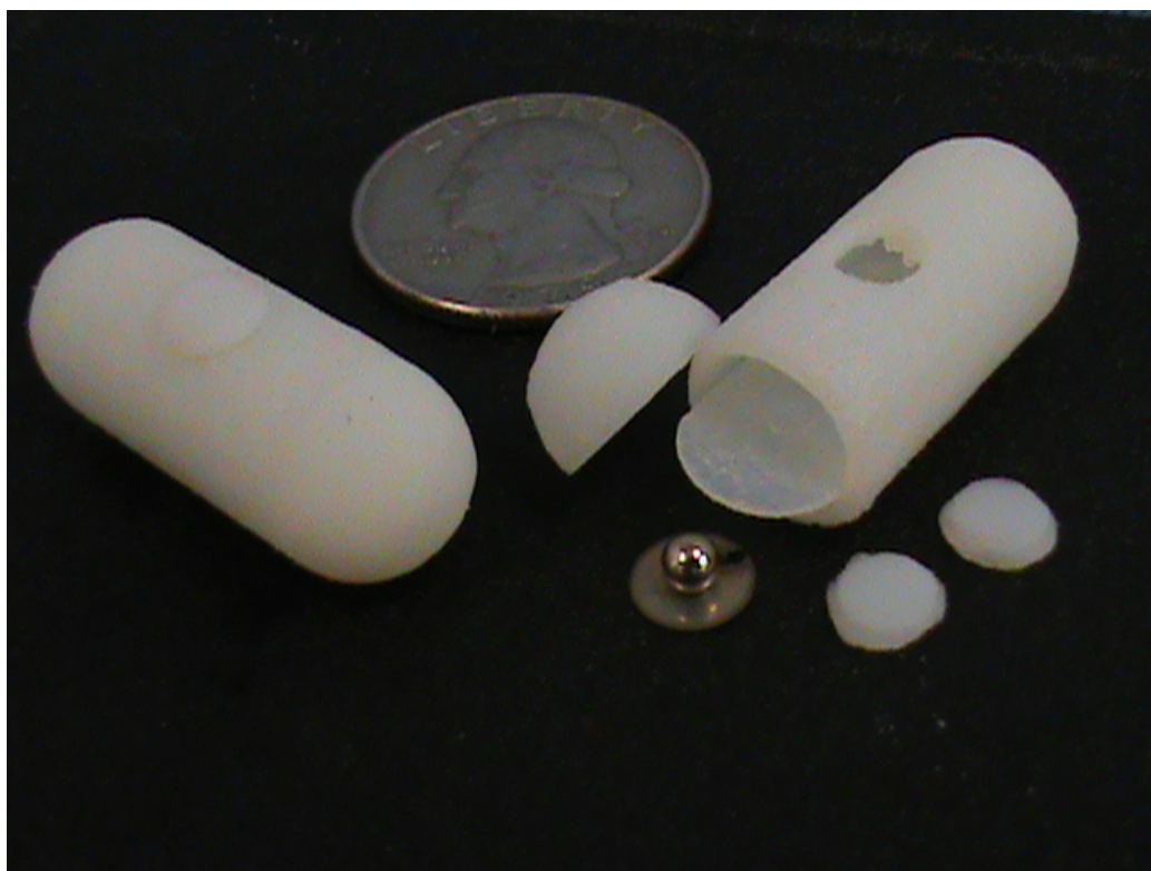
Figure 4.7: First generation IRC prototype (12mm diameter by 32mm length), dividing wall (0.5mm thick), magnetic sphere (3.175mm diameter) and ferromagnetic ring (3.73mm OD, 1.27mm ID, 0.01mm thick).
