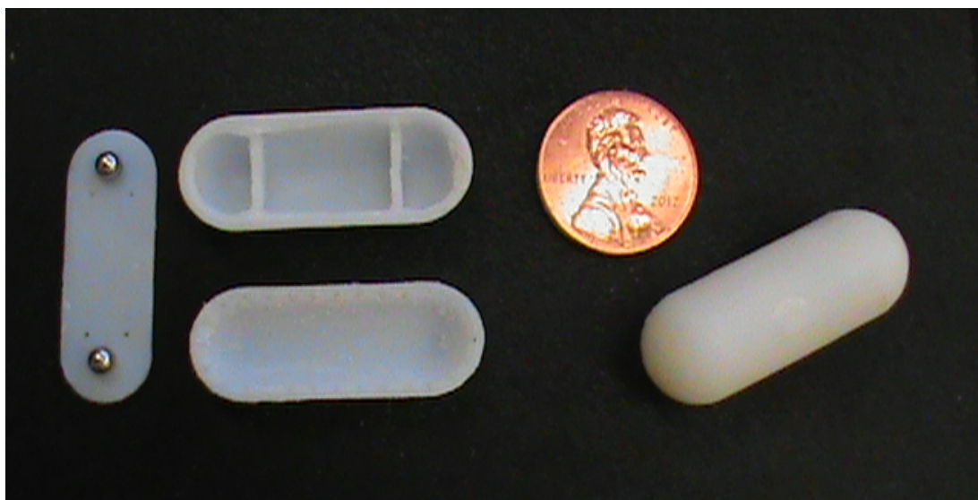
Figure 4.11: Components (left) of third generation Internal Reaction Capsule body (12mm diameter by 32mm in length), dividing wall (1mm thick), magnetic spheres (3.175mm diameter) and ferromagnetic rings, not shown (3.73mm OD, 1.27mm ID, 0.01mm thick) and assembled device (right).
