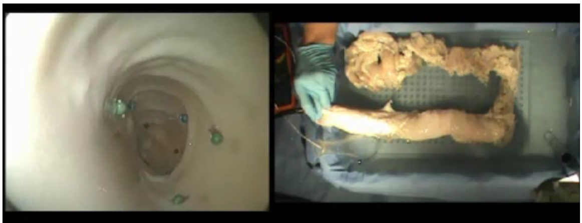
Figure 4.16: Endoscopic view (left) and external view (right) demonstrating the level of visualization provided by three third generation IRCs approximately one minute after a secondary activation.
