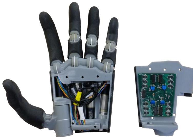
Fig. II-6. Hand with cover removed, showing embedded system and motor units.
