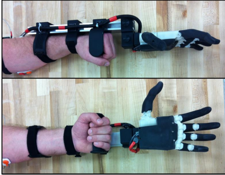
Fig. II-13. Able bodied adapter used in SHAP assessments.
