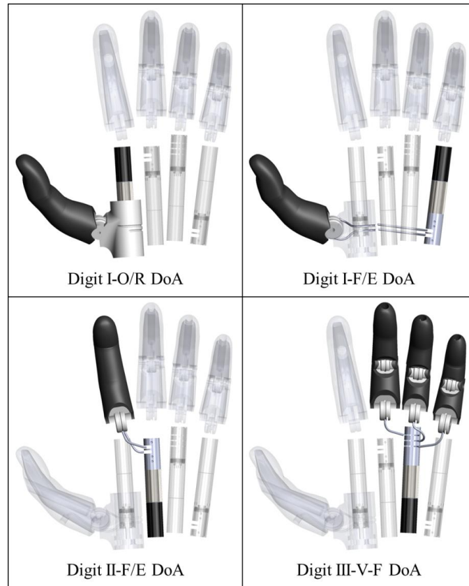
Fig. II-10. First iteration of third generation VMG actuation scheme.
