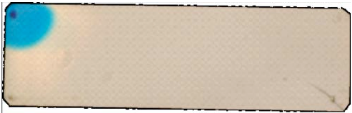
Figure 33. This is an example of what it looks like when the mixing chamber is setup before each experiment with an initial blob of dye. The dye is inserted at the location of the source to be on during the first half-cycle of operation.
