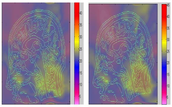
Figure 4.7. Color coded TRE maps superimposed on brain registration results of (a) MLS and (b) TPS. The MLS image has lower maximum and average TRE over the entire image.
