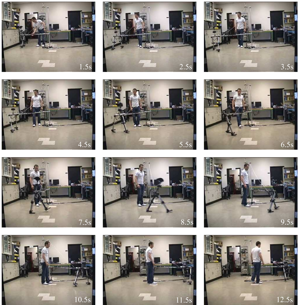
Figure 4.19 Experiment II: Frame sequence of a walking experiment. The walking is characterized with: average forward speed of 0.48\text{m/s} (Froude number Fr = 0.19 ), specific mechanical cost of transport c_{mt} = 0.32 .
