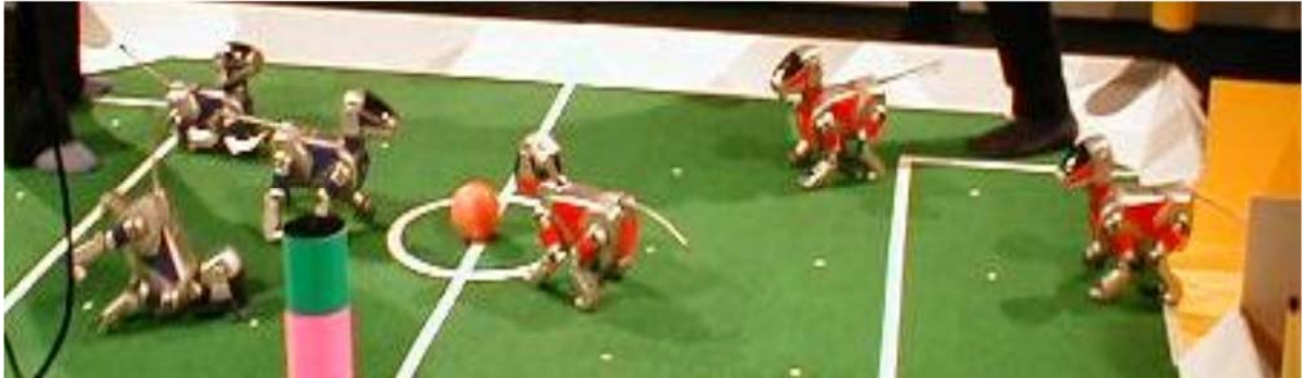
Figure 4.6: Particle filters have been used successfully for on-board localization of soccer-playing Aibo robots with as few as 50 particles.
