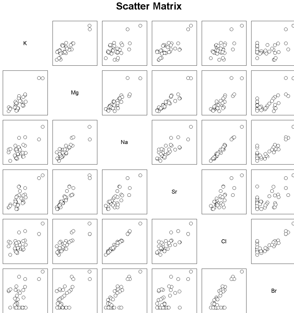
Figure 19. Element correlation matrices for May 2012 groundwater samples. Linear trends between elemental pairs are indicative of conservative elements. Scatter in concentration trends suggests dilution with meteoric water.
