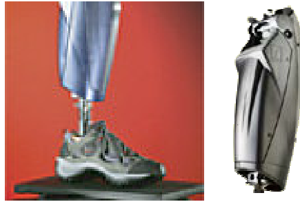
Figure 1-8. Victhom/Ossur “Power Knee” uses electromagnetic actuation and limited battery life.
