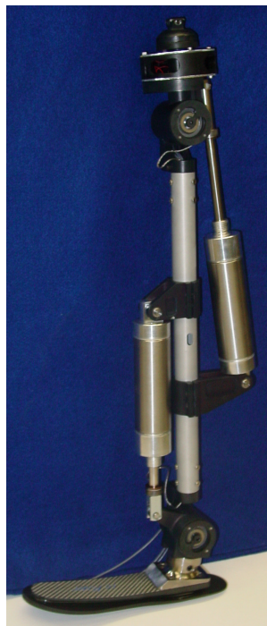
Figure 2-7. Actual tethered transfemoral prosthesis prototype.
