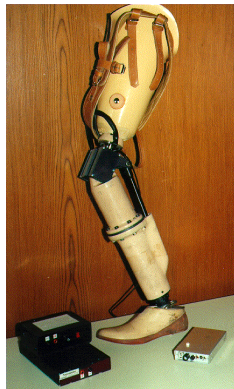
Figure 1-6. Electromagnetically actuated powered knee developed by Popovic with the use of a battery pack.
