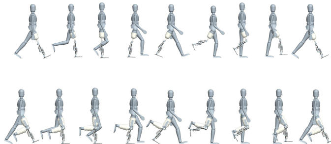
Figure 2-27. Depiction of one stride cycle for transfemoral amputee (above) and healthy subject wearing able-bodied (below).
