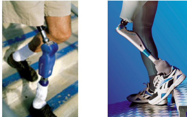
Figure 1-2. The Ossur Rheo knee (left) and the Otto Bock C-Leg (right) represent the cutting edge of microprocessor controlled damping prosthetic knees.
