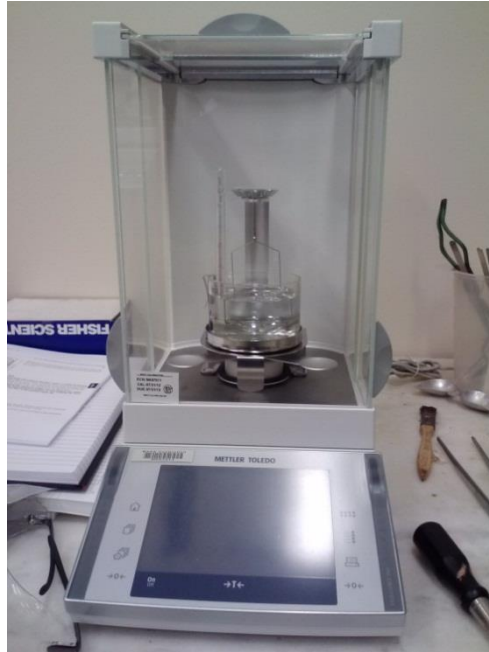
Figure 4.4–1. Mettler Toledo XP204S analytical balance.
