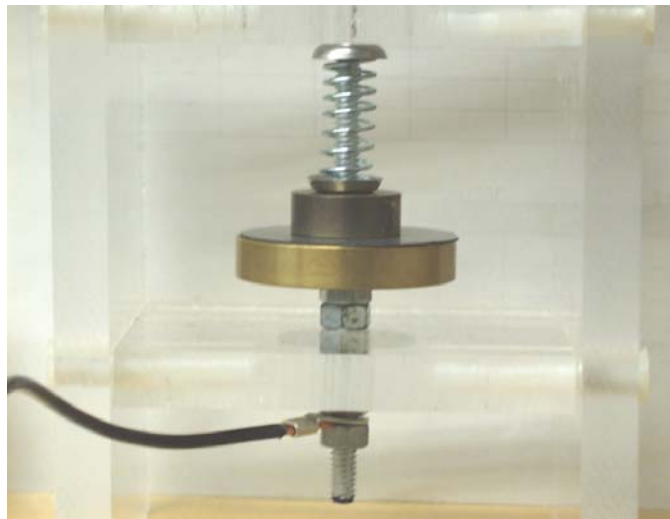
Figure 5.2 Second generation custom test chamber with diamond film sample.
