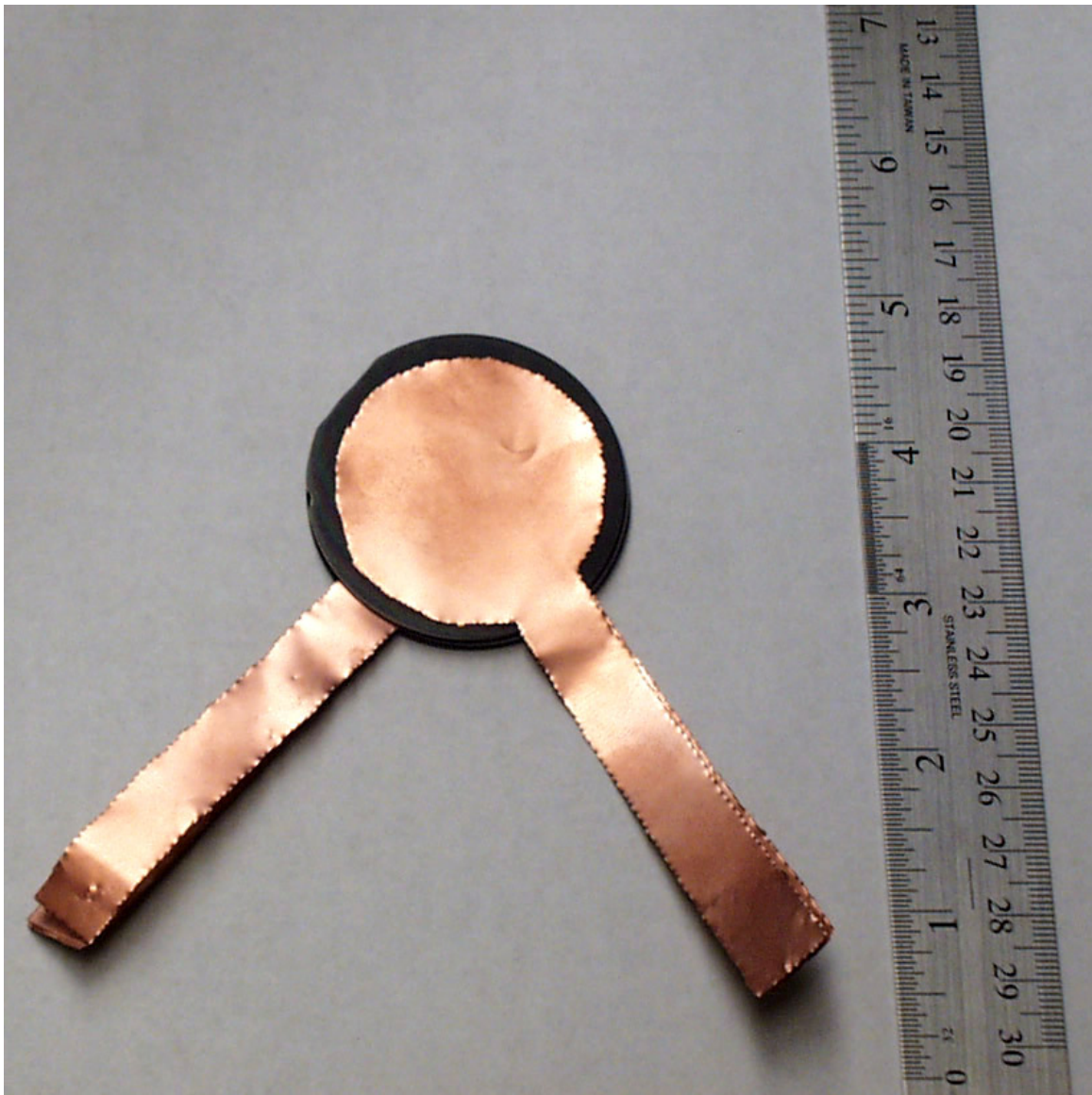
Figure 6.12 Multi-Layered Diamond Capacitor – Overhead View.
