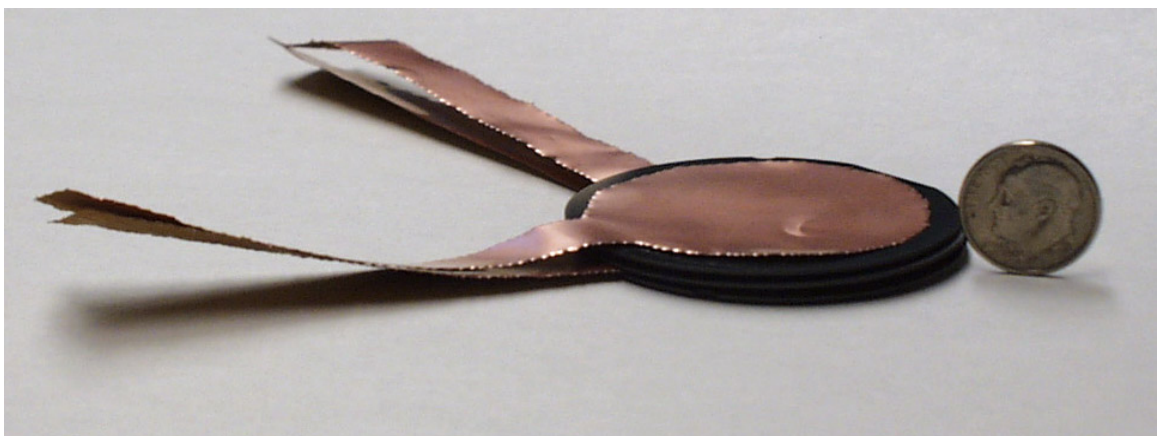
Figure 6. 14 Multi-Layered Diamond Capacitor – Side Profile.
