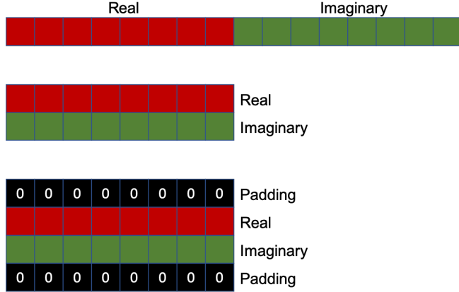
Figure 3.2: Top to bottom: 1D, single-channel convolution. 1D, two-channel convolution. 2D, 1-channel convolution.
