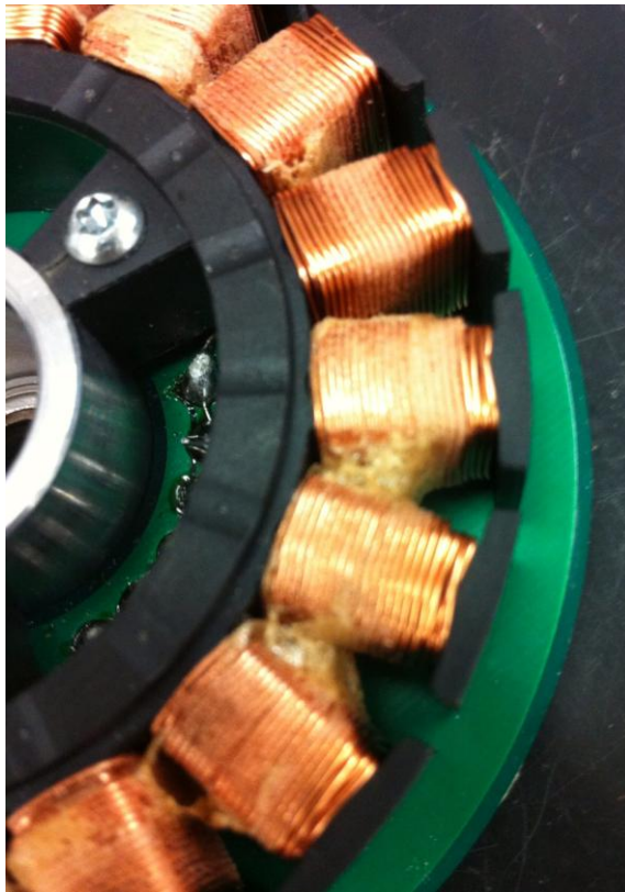
Figure 21: Coil Failure on Old Motor Due to Overheating
