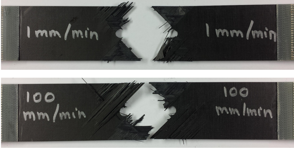
Figure 5.26: Images of Failure from [+45, 0, -45, 90]_{2S} Quasi-Isotropic Open Hole Tension Tests at 1.0 mm/min and 100 mm/min.
