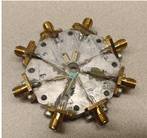
Fig. II-2. High-speed package with eight SMA-connectors and the bonded device. Microstrips connect wires from the device to SMA-connectors. Non-conductive glue is used for attaching connectors and microstrips to the package.
