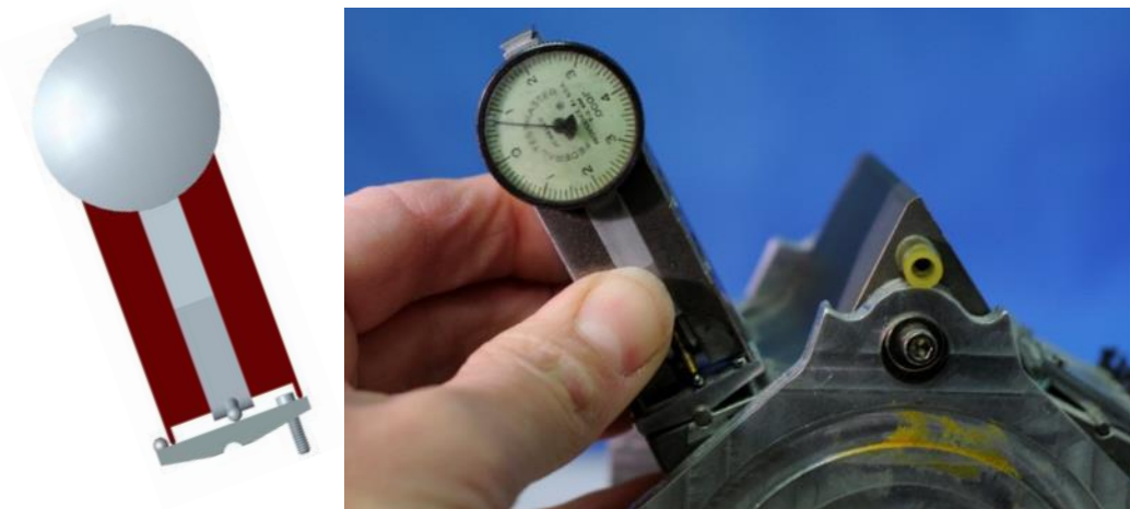
Figure 2-19. CAD model of deflection measurement gauge (left) and gauge in use (right).
