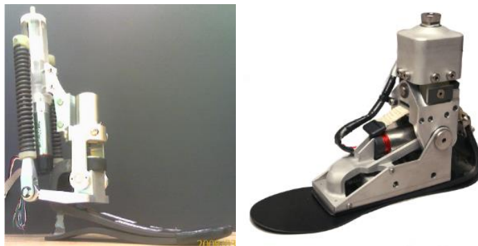
Figure 1-3. Prototype powered ankles developed by Bellman et. al. (left) and Au and Herr (right).
