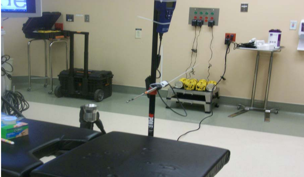
Figure 4 – Anemometer to Measure Air Velocities
