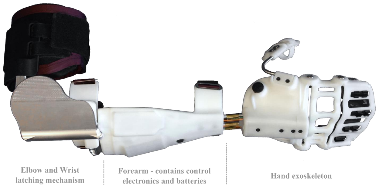
Figure II-12: The Vanderbilt upper-limb exoskeleton. Shown is the integrated hand exoskeleton and semi-passive wrist and elbow orthosis. As indicated, the exoskeleton is composed of three primary segments: the hand exoskeleton; elbow and wrist orthosis latching unit; and the forearm that connects the previous two segments and contains all necessary electronics and batteries.
