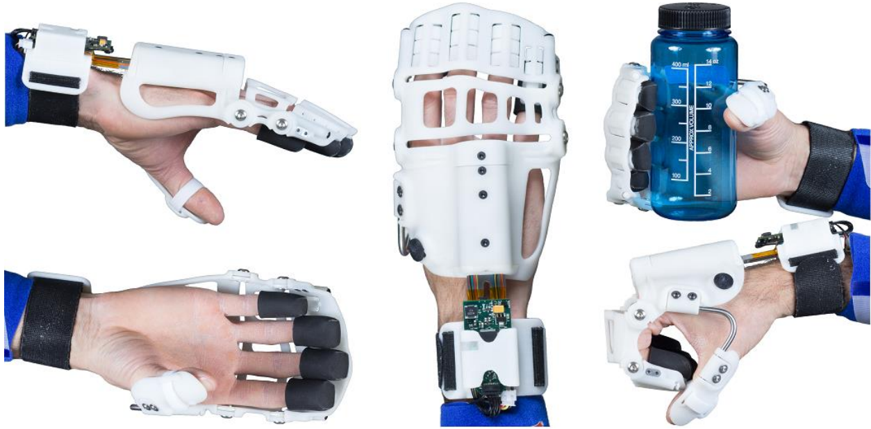
Figure II-1: Hand exoskeleton shown fitted to an approximately 50th percentile male hand.
