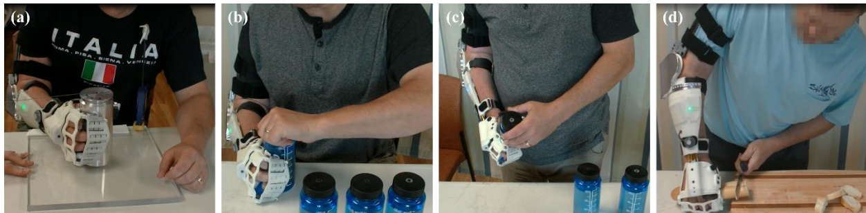
Figure IV-1: Images showing performance of study tasks. (a) shows a subject engaged in the grasp strength test with the large grasp cylinder, (b) is the sitting bottle opening test, (c) standing bottle opening test exhibiting no use of the table or other support, (d) shows a subject cutting bread while using the exoskeleton.
