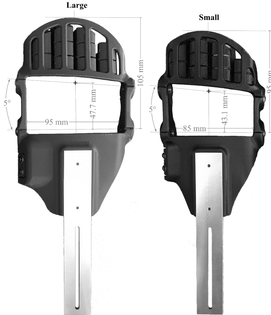
Figure II-10: Hand fit shells showing Large and Small dimensions. Hand shell dimensions are based on a middle finger length and MCP to PIP distance estimated at 50% and 23%, respectively, of the overall hand length. Large shell is consistent with a 90 th percentile male hand and the small with a 95 th percentile female (15 th percentile male) hand.
