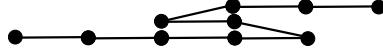
Figure V.1: An Ideal Chain The simple model of an ideal chain can be used to calculate the entropic forces in one dimension. This image represents just one possible microstate that this ideal chain can inhabit.
