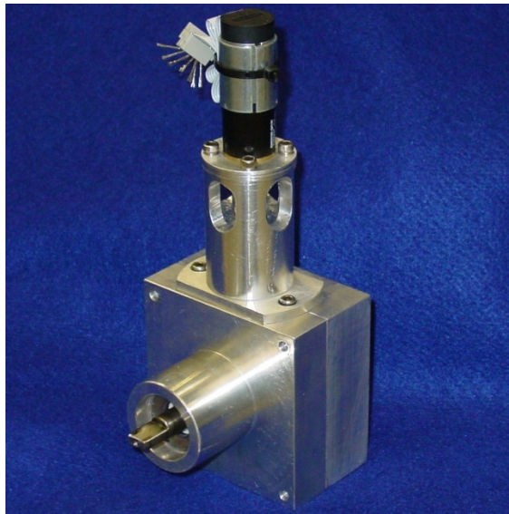
Fig. 2-14. VDVP prototype (with a DC motor assembled).
