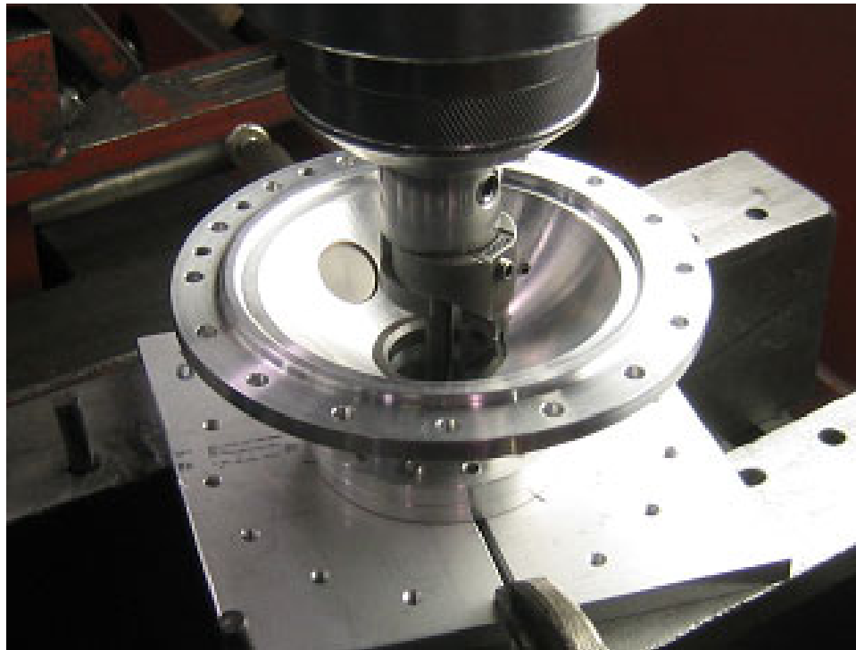
Figure 4-8: Cutting the Valve Seat.
