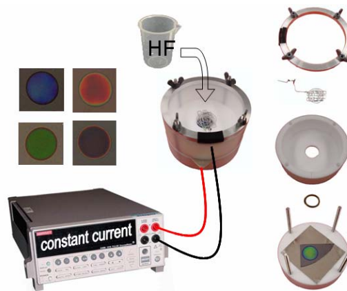
Figure A.1. Etching cell assembly, its electrodes connection with current source, and the resulting porous silicon samples after etching (Figure courtesy of Ph.D. dissertation of Sharon M. Weiss, University of Rochester, 2005).
