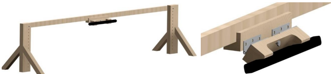
Figure 2-11: Design of the Eye-Tracker Mount
