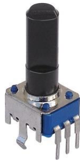
Figure 3-8: Potentiometer Used for Measurement of Rotational Subsystem
