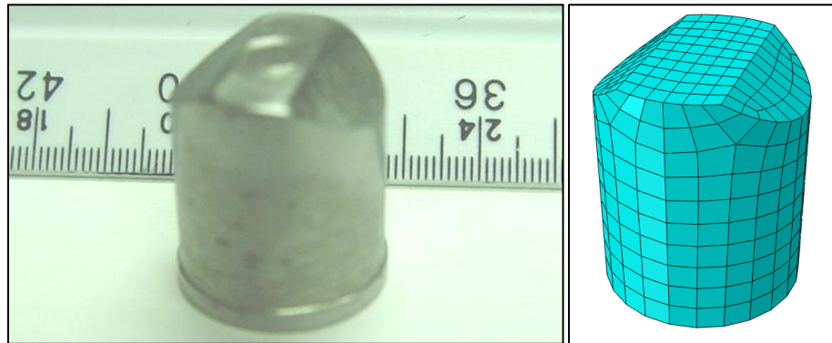
Figure 7.12 MIL-P-46593A Standard 0.50 Caliber FSP (left) and model (right)
