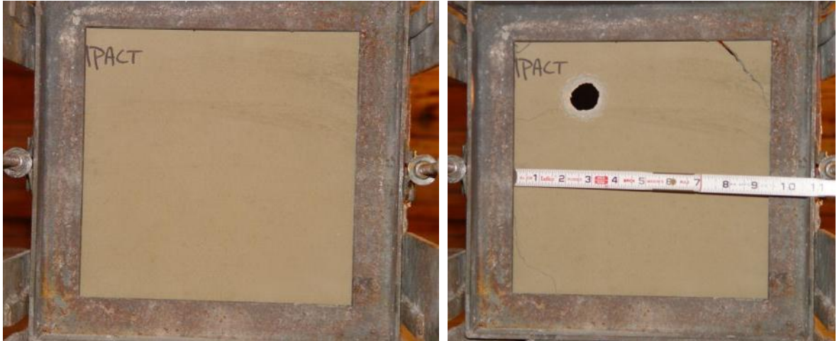
Figure 7.13 Ashcrete target panel before (left) and after (right) impact
