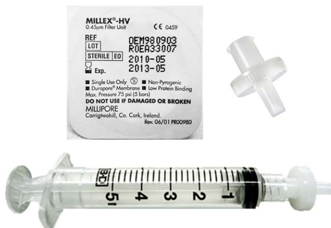
Figure 43. Configuration of medium filtration system; Millex-HV syringe filter, 0.45 µm, PVDF, 13 mm, ethylene oxide sterilized
