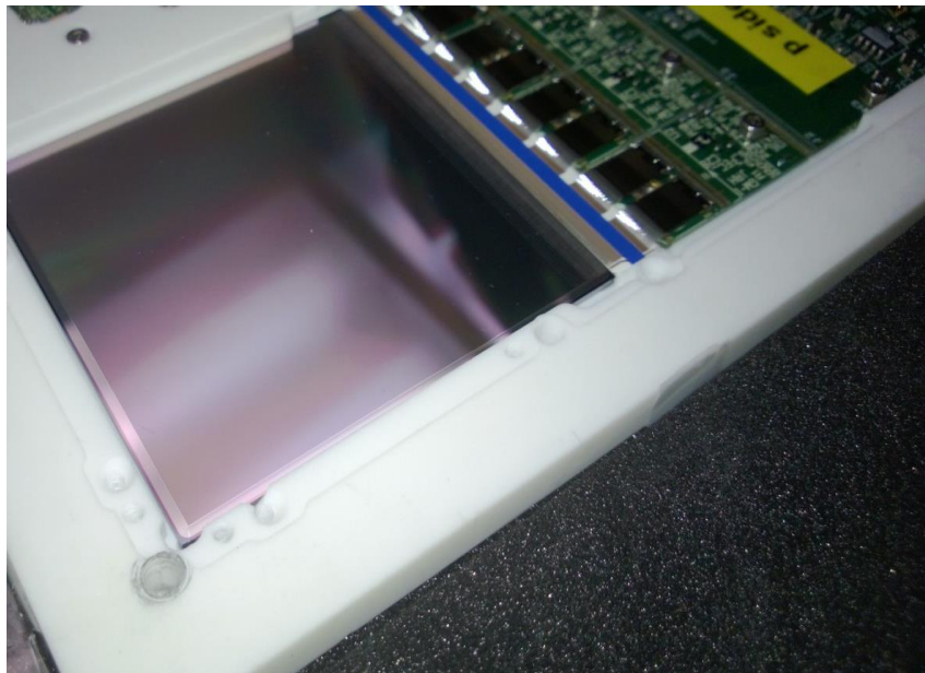
Figure 9. Si detector active area showing 1024 strips
