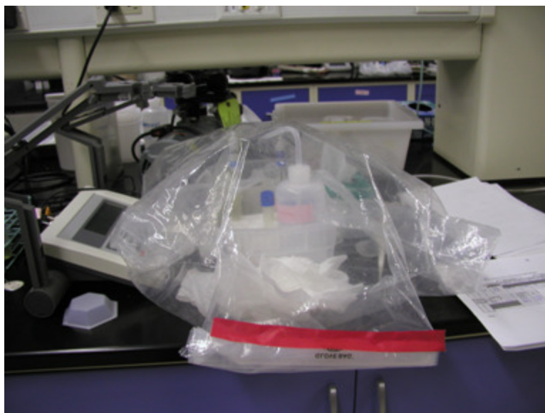
Figure 16. Glove bag filled with nitrogen for external pH and Eh readings for the oxidation/reduction experiments using an electrolytic technique.
