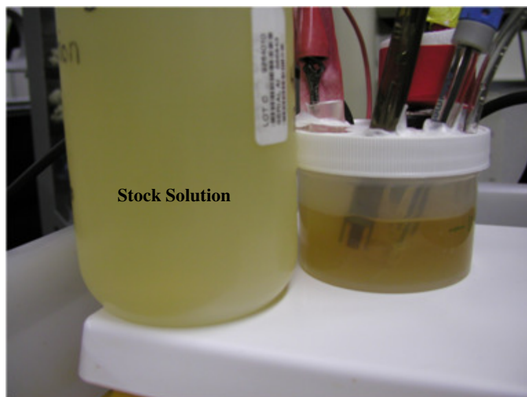
Figure 23. Color change of electrolytic solution after applying a potential of -1200\text{mV} in comparison to the 0.01\text{M} iron(III) nitrate stock solution.
