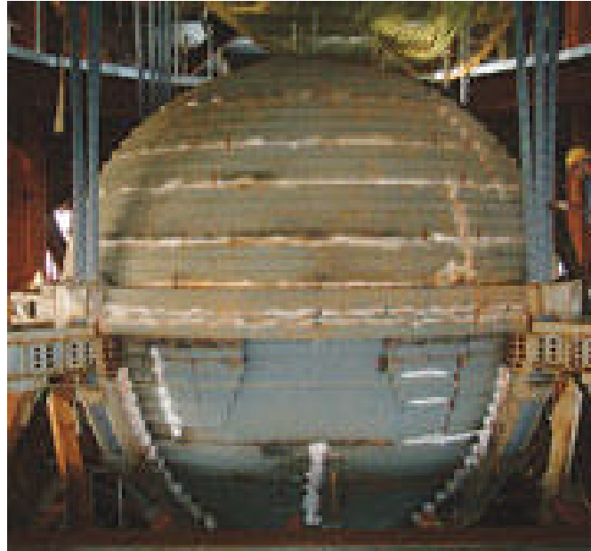
Figure 5. 800 ton steel sphere used in the passive mass damper
