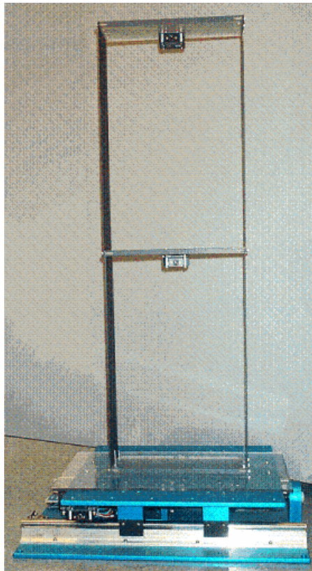
Figure 18: Two-story building used for experiments
