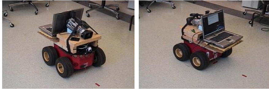
Fig 5.5 Mobile robot Skeeter with camera and laptop
