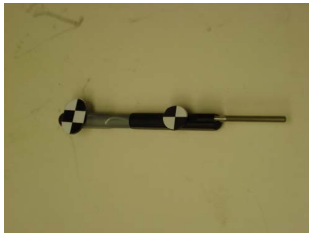
Figure 3: The probe surgical tool. The probe is used to localize fiducial points.
