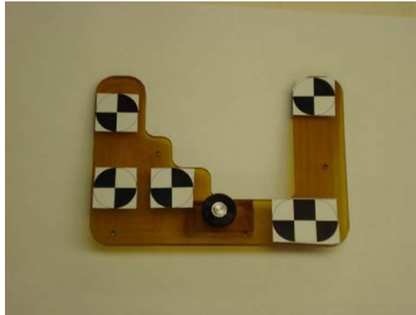
Figure 9: The coordinate reference frame. The CRF is used to account for movement of the target and the tracker during the tracking process.
